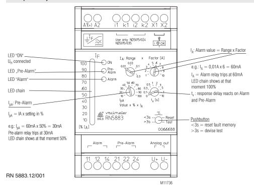
It is of advantage to keep the range small and the Factor high. Example: Setting 300 mA: Range 0,1 x Factor 3 = 300 mA
